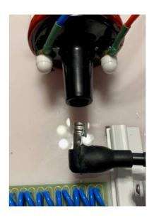
3. Finally, remove the coil plug from the red coil. This clips in firmly and should be refitted the same way. Once all 3 connections are removed, the complete spark gap assembly will slide out easily for cleaning.
