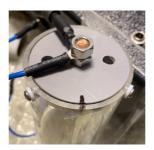
Do **NOT** tighten the screws too much! Only tighten them until it stops – do not over tighten.
