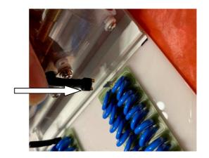
2. Remove the spade clip from the capacitor board and the second spade clip from the second capacity board behind this (as seen in the picture above). Only remove these 2 clips.
